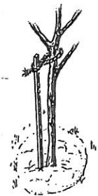
single staking for small trees (up to 1" diam.)
